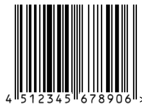
Figure 5-1 EAN-13 (example of EAN/UPC Symbology)
