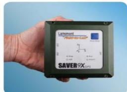
The SAVER™ 9X30 is a self-powered field data recorder with an internal triaxial accelerometer, and six externally configurable channels. The 9X30 is provided with temperature, humidity and atmospheric pressure sensors and can be optionally configured with onboard GPS logging capability. Powered with 9V lithium batteries, the instrument and will operate continuously for up to 30 days.
